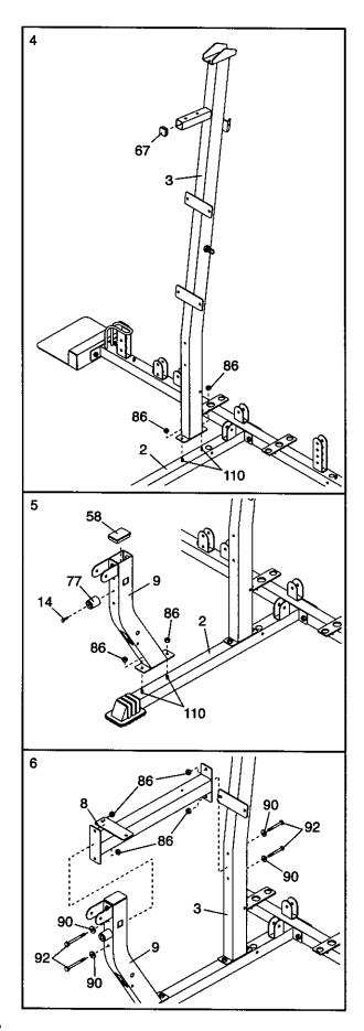
Press a 2" x 3" Inner Cap (58) into the top of the Squat Upright (4). Slide the Squat Upright onto the two indicated 5/16" x 2 1/2" Carriage Bolts (110) in the Long Base (120). Finger tighten a 5/16" Nylon Locknut (86) onto each Carriage Bolt. Do not tighten the Nylon Locknuts yet.
